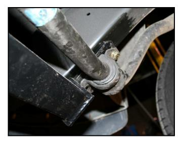
Apply Loctite. Install (**snug**, **not tight**) four of the supplied **17mm** bolts with washers to re-secure the sway bar and SBS to the frame, while allowing for final mounting position to be fine tuned.
