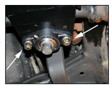
Remove the set screws and apply LocTite.
