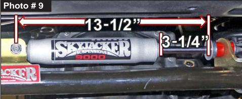
Cycle steering from side to side & check for adequate clearance.
