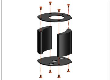
on the upper plate line up with the clearance holes on the lower plate.
