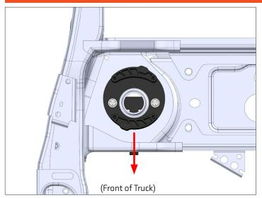
Ensure the upper bracket is in the orientation shown before installing the bolts.
