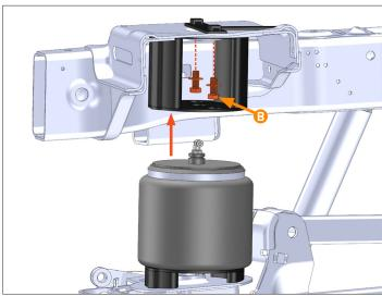
3 Re-install the two 1/2" bolts with some threadlocker and torque to **75 FT.LB.**
