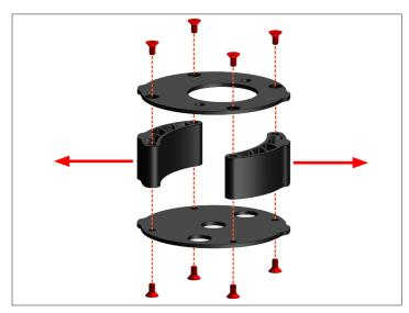
Using a 3/16" hex socket, un-bolt the 8 fasteners holding the upper bracket together. Discard the fasteners.
