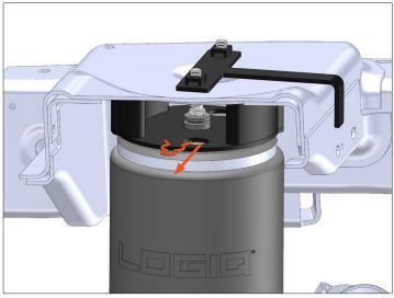
Fully deflate air springs and disconnect air line from the elbow air fitting. Remove the hairpin clip from the air spring. Retain the hairplin clip for re-installation.
