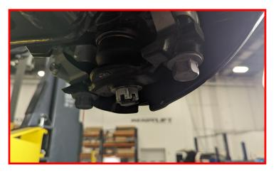
Loosen but do not remove the (4) top strut nuts.
