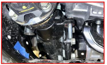
Assemble ReadyLIFT rear differential mount as shown.
