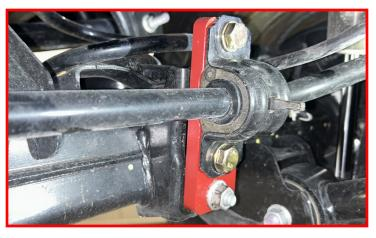
Install the brake line drop bracket into the factory location using the factory hardware.
