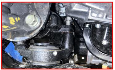
Raise the differential back up to allow the removal of the rear diff mount.
