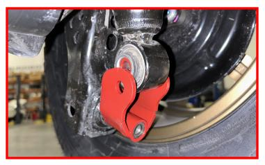
Using the supplied M12 x 30mm hex head bolt, M12 washers and locking nut, install the support tab through the factory shock mount.
