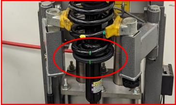
Install the ReadyLIFT front strut spacer onto the top of the strut.
