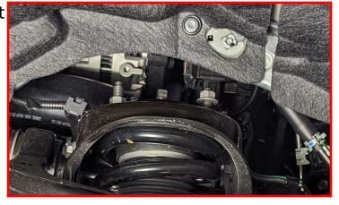
Remove the sway bar bolt from lower control arm.
