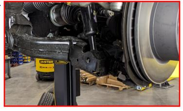
Install the factory lower shock bolt. **DO NOT TIGHTEN AT THIS POINT.**
