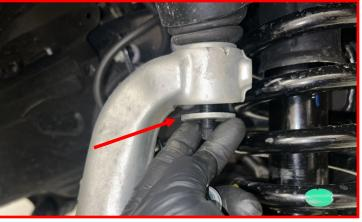
Install the supplied M12 flange nut onto the ball joint.
