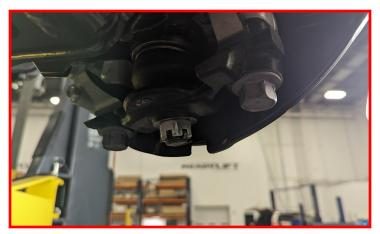
Install the sway bar using the factory hardware.
