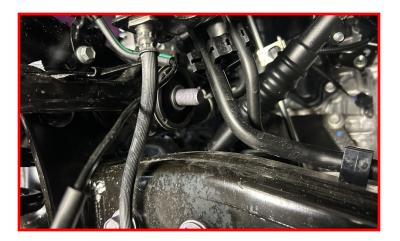
When removing the left (driver) side upper control arm pivot bolt, you will notice that the bolt will make contact with the intercooler/ boost tube.
