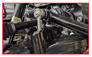
Guide the lower strut mount into the lower control arm pocket.
