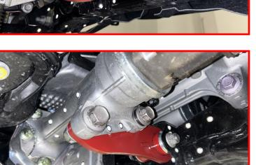
Install the supplied M16 locking nuts and washers.
