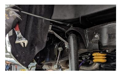
Remove the bolt holding the brake line bracket to the axle.
