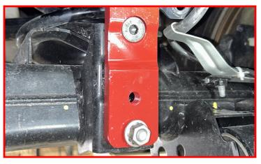
Install the supplied M12 washer and locking nut onto the backside of the factory sway bar mount.
