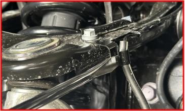
Remove the wire from the bracket.
