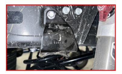
Install ReadyLIFT rear bump stop extension using the provided M8 X 70mm bolts, M8 washers and thread locker.
