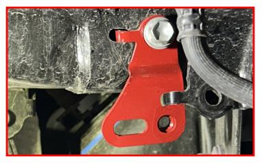
Install rear brake line bracket onto the brake line drop bracket using the supplied M8 x 20mm, M8 flat washer and thread locker.
