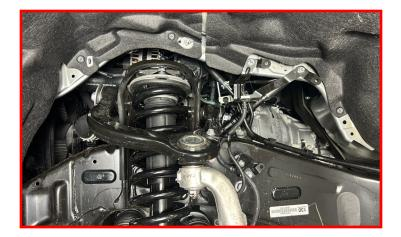
Use a flat blade screw driver or similar tool to pry the (3) upper control arm ABS brackets open.
