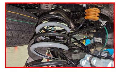
Remove the isolator from the spring. And install isolator onto ReadyLIFT spring spacer.
