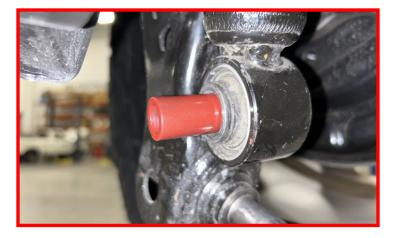
Install ReadyLIFT rear shock extension onto axle.
