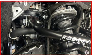
Install the upper control arm ball joint into the knuckle in the factory orientation.
