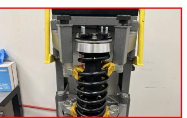
NOTE: During this process, ensure that the spring does not rotate relative to the lower spring perch.
