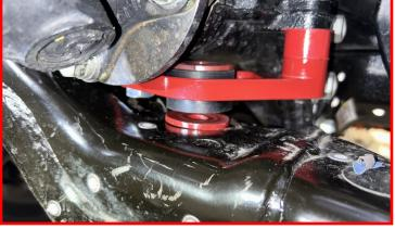
Install the supplied M14 x 40mm hex head bolt, flat washer, 3/8" thick laser cut washer and thread locker through the crossmember and into the rear diff drop.
