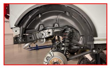
Prior to installing wheels, complete all installation steps on the opposite side. Install the wheels and lower the vehicle to the ground. Torque the lug nuts to the wheel manufacturers specs. Jounce the vehicle to settle the suspension to the new ride height.
