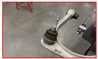
Using the appropriate tool included in the ball joint press, orient the ball joint so the flats match up and slowly press the ball joint into the supplied upper control arm.
