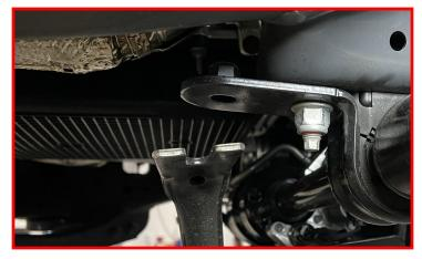
Tighten the (2) forward sway bar skid plate bolts.
