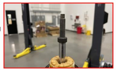
Remove the seal head bump cap.
