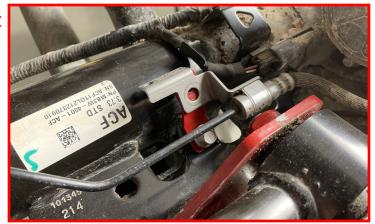
Install the factory brake line bracket to the supplied brake line relocation bracket using the supplied M8 x 20mm hex head bolt, washers and locking nut.
