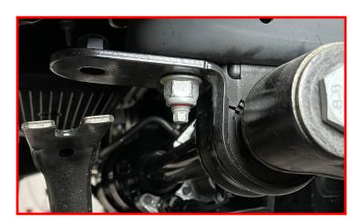
Lower the sway bar down and back to aid in removal of the rear lower control arm pivot bolt.
