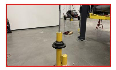
Install the seal head bump cap.
