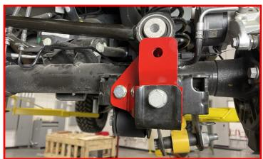
Install the supplied rear brake line bracket on to the axle mounting point using the factory hardware.
