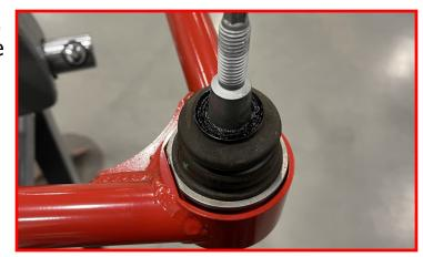
Install the factory ball joint retaining clip.
