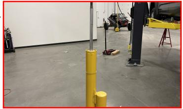
Install the preload collar over the strut body. Ensure the collar is completely seated on the retainer clip.
