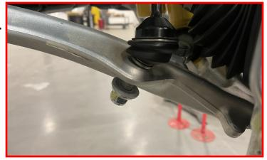
Raise the sway bar back into the factory orientation.
