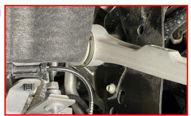
When installing the driver side upper control arm you will need to disconnect the steering linkage.
