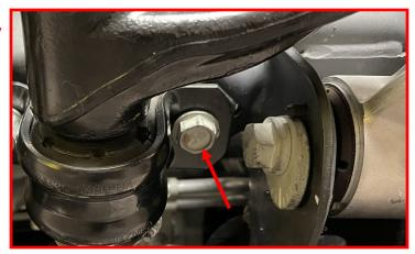
Install both the driver and passenger rear sway bar skid plate bolts.
