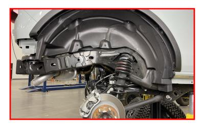
With the rear wheels removed, locate and remove the (12) mounting clips and the (3) mounting screws that hold the rear fender liners in place.
