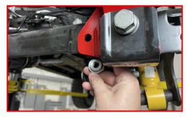
Install the supplied M14 x 30mm hex head bolt, locking washer and flat washer through the rear track bar bracket and into the rear track bar bracket nut
