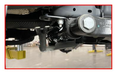
Remove both the driver and passenger forward sway bar retainer cap bolts.
