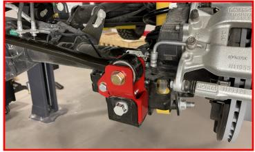
Using an appropriate jack, support the axle.
