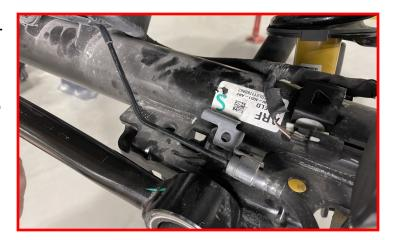
Install the supplied rear track bar bracket in the factory location.
