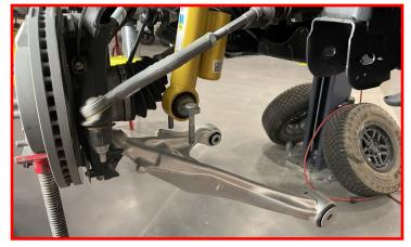
Remove the (3) top strut nuts and carefully remove the strut assembly from the vehicle.
