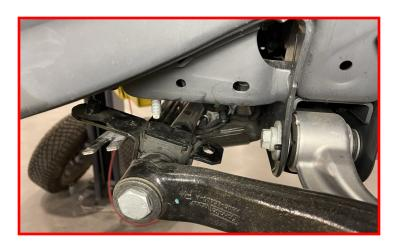
Install the driver and passenger rear sway bar retainer cap nuts.
