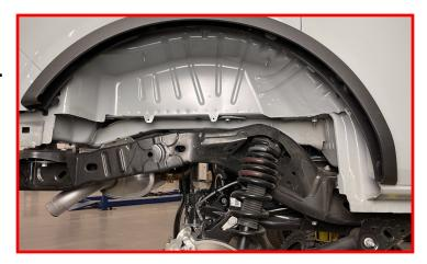
To aid in the removal and installation process, it is best to loosen the rear track bar at the axle.
