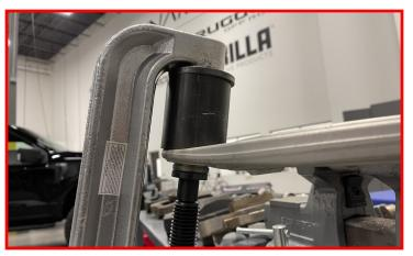
Remove the ball joint from the factory upper control arm.
