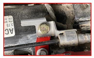
Install the rear track bar into the track bar bracket using the supplied M16 x 90mm hex head bolt, washers and locking nut.
