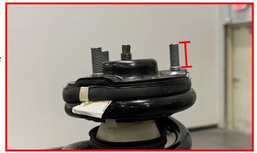
Install the top strut spacer (68-21300FSS) onto the strut assembly using the factory nuts.
