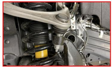
Remove the upper control arm pivot bolt.
