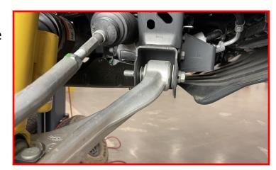
Install the factory alignment cam plate over pivot bolt and then install nut.
