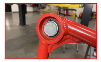
If removed, install the factory ball joint boot.
