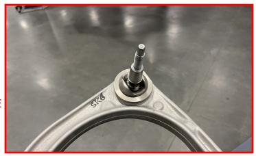
Using a ball joint press and the provided tube and washers, press the ball joint out of the factory arm.
