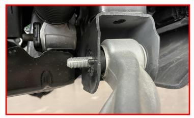
With the lower control arm pivot removed, Swing the lower control arm down while removing the lower strut studs from the control arm.
