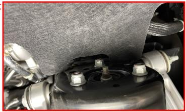
Remove the lower strut nuts.
