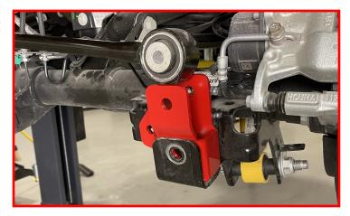
Install the factory hardware through the factory track bar mount and the track bar bracket.
