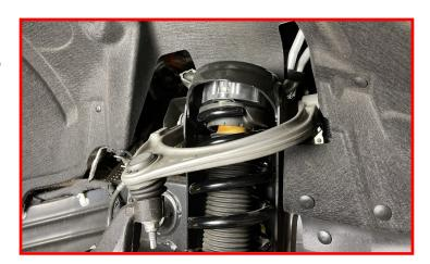
Raise the lower control arm up and guide the lower strut studs into place.
