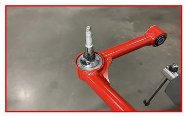
Install the provided upper control arm dust cap. Ensure the "R" is facing towards the outside of the vehicle.
