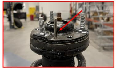
Place the strut into a spring compressor. Mark the top hat to spring location.
