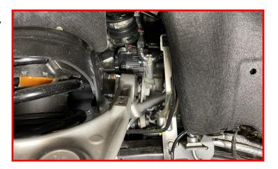
With the upper control arms out of the vehicle, remove the retaining clip on the top of the ball joint.
