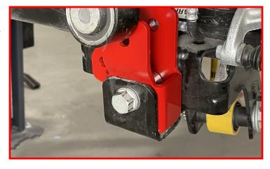
Install the supplied rear track bar bracket nut into the hole located in the factory track bar bracket.
