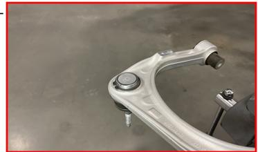
Using a flat head screw driver, carefully remove the OE ball joint boot.
