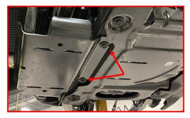
Install the single retaining rivet that secures the inner fender liner.
