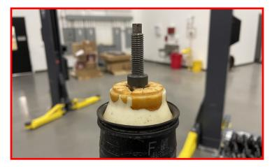
Compress the spring enough to install the factory top hat. Being sure to keep the strut body and upper spring isolator in the factory location, rotate the factory top hat 180 degrees from the previously made marks. This will orient the spring in its original location to prevent the spring from bowing. Install the factory strut shock shaft nut. When tightening, make sure the top of the strut shaft is fully seated into the top hat.
