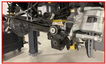
Remove the factory brake line bracket located on the axles right (passenger) side in front of the track bar bracket.
