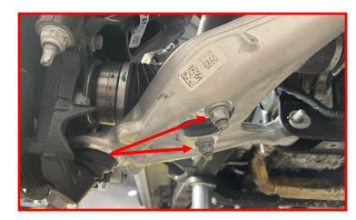
Loosen but do not remove the (2) forward sway bar skid plate bolts.
