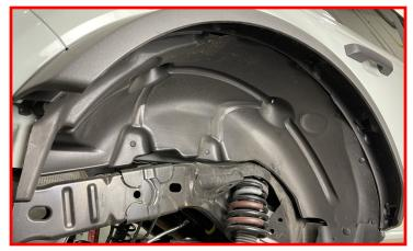
Remove the rear fender liners.
