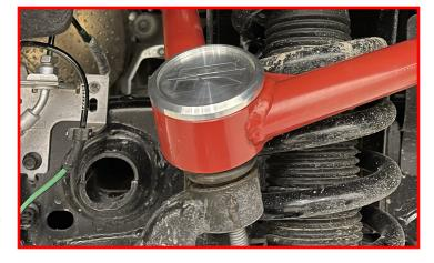
Install the pinch bolt on the top u-joint.
