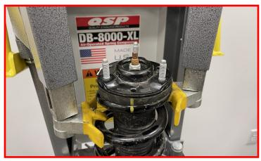
Before install the top strut spacer you will need to trim the factory top hat studs to make clearance for the strut spacer.
