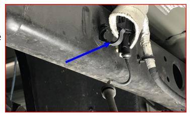
Support the axle with a suitable jack. Remove both Driver and Passenger shock bolts from the vehicle.
