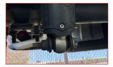
Install the rear wheels and lower vehicle to the ground. Torque the lug nuts to the wheel manufacturer specs, the lower shock hardware to 66-ft/lbs and u-bolts to 110-ft/lbs. Attach the vehicle negative power source. Have the alignment set to the recommended specs at the end of the instructions.
