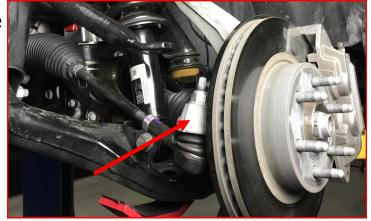
Install the axle nut. Torque to 185 ft-lbs.
