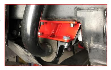
Install the lower sway bar end link to the control arm and sway bar. Torque to 35 ft-lbs.
