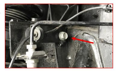
Remove the lower sway bar end link from the control arm and sway bar.
