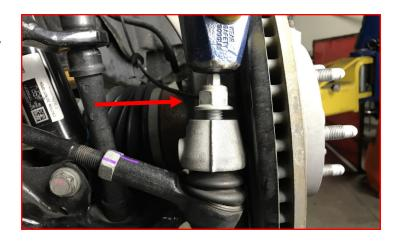
Remove the ABS sensor harness from the knuckle and hang out of the way.
