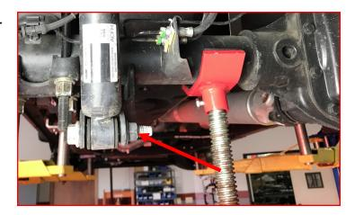
The rear dampers are etched with the appropriate corner.
