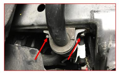
Install the sway bar drops to the frame using factory hardware. Torque to 45 ft-lbs. Install the sway bar to the drop brackets using M10 bolts, washers and M10 nuts. Torque to 45 ft-lbs.
