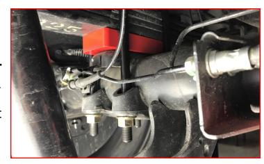
Install the shocks using the factory hardware. Do not tighten at this time.
