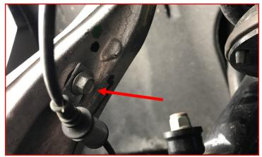
Remove the brake line bracket from the frame. Be sure to retain the factory hardware.
