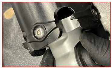
Install the completed rear damper assembly into the vehicle using the factory mounting hardware.
