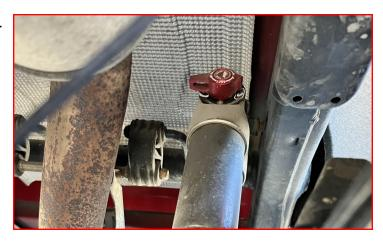
Loosen but do not remove the u-bolts on the passenger side. Completely remove the u-bolts on the driver side and discard. Lower the axle enough to install the ReadyLIFT block. Raise the axle while lining up the center pins on the axle and block. Install the provided u-bolts. Do not fully tighten at this time. Repeat for the other side of the vehicle.
