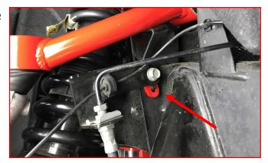
Install the ABS sensor harness back to the knuckle.
