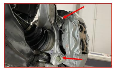
Remove the factory brake line bracket from the chassis.
