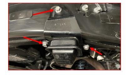
Using factory hardware, install the supplied end link bracket to the frame.
