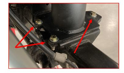
Install the air spacer nut. Ensure the boss is seated in the slot on the air lift spacer.
