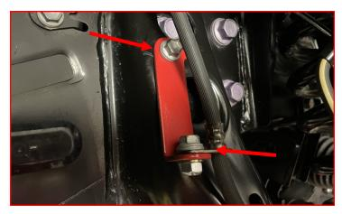
Attach the ABS wire to the strut perch using factory hardware.
