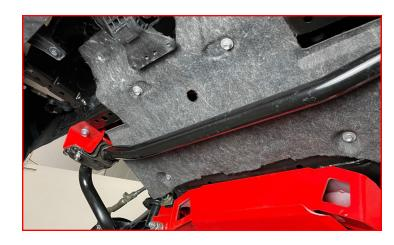
Trim the front air dam 0.25" from the inner edge. Contour the line to blend it into the air dam.
