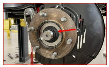
Using factory hardware, insert the upper control arm ball joint into the knuckle. Rest the knuckle on the knuckle adaptor/steering stop.
