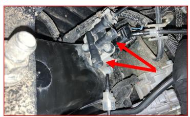
Remove the factory nut on the bottom of the air bag.
