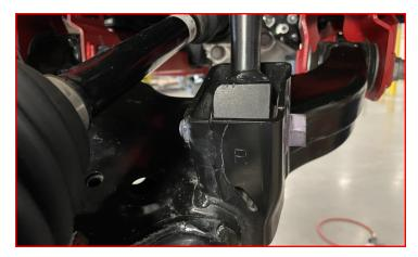
Remove the four (4) factory bolts holding the knuckle to the hub.
