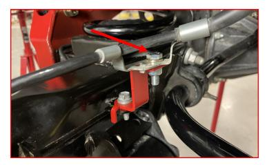
Install the rear ABS relocator between the brake lines and the axle using the factory bolt holding the brake line to the axle.
