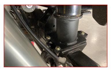
Slide the Air Bag Spacer Plate between the axle housing and the bag mount on the axle housing. Install the 3 supplied M10x40mm bolts, washers, and lock nuts.
