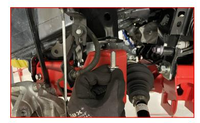
Feed a ratchet extension up through the lower mounting hole to tighten the bolt.
