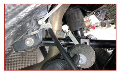
Mate the air ride sensor link to the new sensor relocation bracket using the factory nut. Torque to factory spec.
