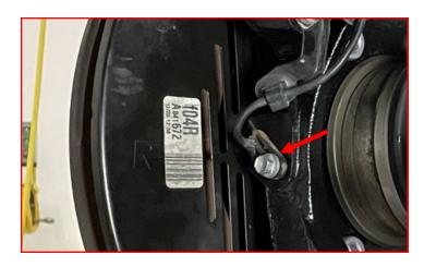
On the factory dirt shields removed on page 8, remove the retaining clip for the sound deadening in the front lower corner.
