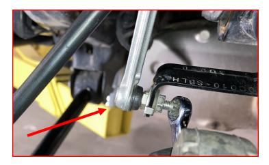
Remove the rubber isolator from the upper control arm. Save the factory hardware and rubber isolator.
