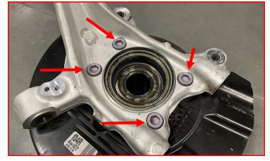
Carefully remove the dust seal off of the back of the knuckle. Using a flathead screwdriver or similar tool, carefully work around the outer edge of the seal to release it from the knuckle.
