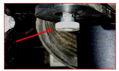
Remove the Ride Height Link from the tab on the upper control arm.
