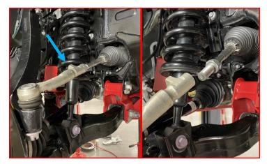
Note how the <u>nub</u> on the tie rod is opposite of the factory location in the previous step.
