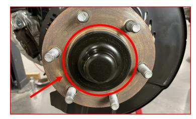
Remove the cotter pin, sleeve, and nut.
