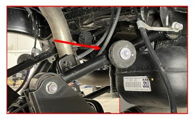
Using the factory hardware, install the Air Sensor Relocation Bracket sandwiched between the rubber isolator and upper control arm.
