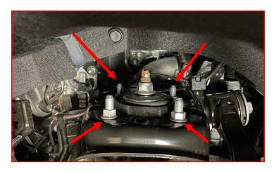
Loosen but **DO NOT** remove inner control arm nuts.
