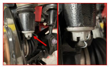
Remove the two (2) nuts holding the brake line bracket to the body (driver shown in the left image, passenger shown in the right image).
