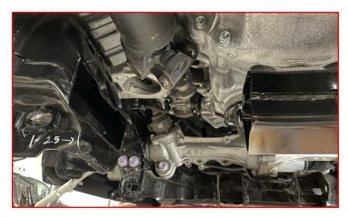
Temporally install the rear crossmember with the differential mount on the driver side. Use the supplied M18-2.5 X 160mm hex heads bolts and cam block off plates (four total).
