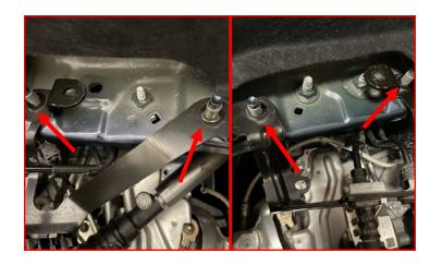
Remove the driver side brake lines from the plastic clip on the inside of the body panel opposite of the bracket removed in the previous step (left image).
