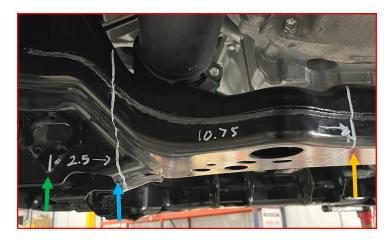
Using a suitable cutting tool, cut the crossmember at the marked lines.
