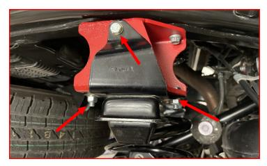
Attach the supplied rear shock to the lower mount using factory hardware.
