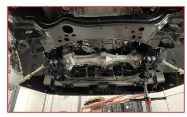
On the backside of the rear crossmember, mark a vertical line 2.5 inches from the **center** of the left hand side alignment cam hole.
