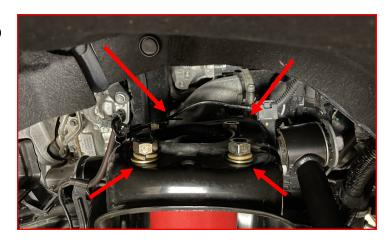
Raise the lower control arm enough to insert the factory lower strut bolt and nut. Install from front to rear.
