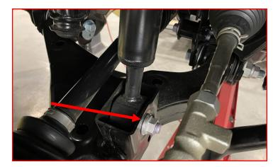
Loosen but **DO NOT** remove the four (4) upper strut bolts.
