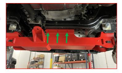
Remove the factory front differential vent hose. **Retain factory hardware.**
