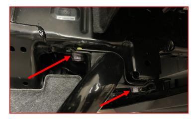
Remove the ABS wire bracket on the upper control arm and strut perch.
