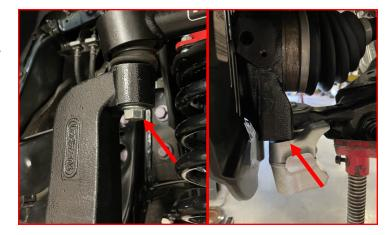
Apply a small amount of medium duty thread locker to the factory lower ball joint bolts.
