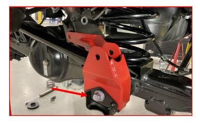
Using the supplied M12-1.75 X 35mm hex head bolt, M12-1.75 locking nut, and two (2) M12 washers attach the Panhard bar bracket to the factory upper control arm bracket.
