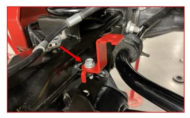
Using the supplied M8-1.25 X 20mm hex head bolt, M8-1.25 locking nut, and two (2) M8 washers attach the brake line to the supplied bracket.
