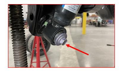
Remove the upper shock nut and bushing.
