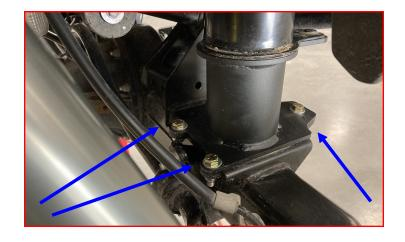
Torque the air bag spacer nut to 18 ft-lbs.
