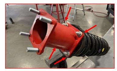
Install the strut and spacer assembly into the vehicle using the supplied 7/16-20 serrated flange nuts.
