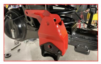
Using factory hardware, attach the bracket to the axle in the factory mounting location.
