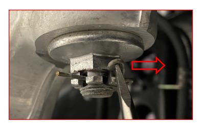
Loosen but **DO NOT** remove the upper ball joint nut.
