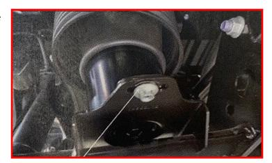
Gently compress the air bag and slip the air bag spacer between the bottom of the air bag and the top of the bag mount on the axle housing.
