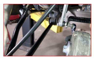
Using an air nozzle or similar, slowly add some air to the bags via the disconnected hose at the manifold. As bag inflates, check alignment of bag with bottom spacer and top bag mount on the frame. If aligned, continue to fill the bag with just enough air to put pressure between the fame and axle mounts. Quickly remove the nozzle and insert the line back into the manifold.
