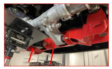
Install the rear crossmember using he supplied M18-2.5 X 160mm hex head bolts, M18-2.5 locking nuts, and M18 flat washers,
