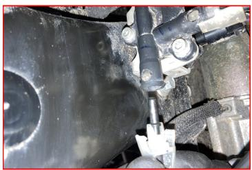
With pressure in the bag, torque the three lower M10 bolts to 45 ft-lbs.
