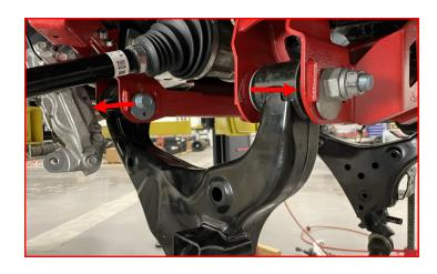
Remove the factory bump stop from the chassis mount.
