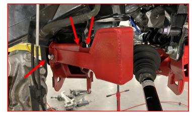
Use a supplied M10-1.25 X 25 hex head flange bolt to attach the bump stop to the chassis.
