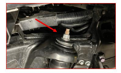
Remove the two air lines from the manifold located on the right rear frame rail.
