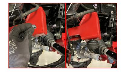
Attach the front strut spacer to the factory strut using factory hardware.
