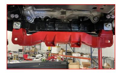
Raise the front differential and install the to the front crossmember using the factory front differential mounting brackets and hardware.
