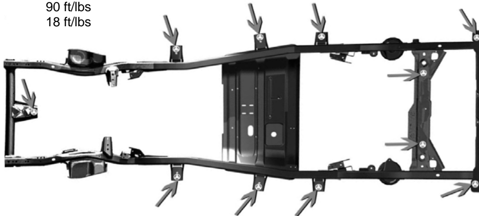
DIAGRAM 1 (SHOWING LOCATIONS OF BODY MOUNTS)
