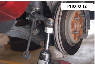
15. Loosen the upper ball joint nut as shown with a 18mm wrench. Do not totally remove the upper ball joint nut at this time. Using a hammer slightly tap the upper tie rod mount to loosen taper. **See Photo 13 & 14.** Position knuckle to allow for strut removal.
