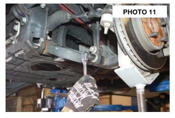
14. Remove the tie rod from the knuckle as shown using a 21mm socket/wrench. See Photo 12. Retain hardware.
