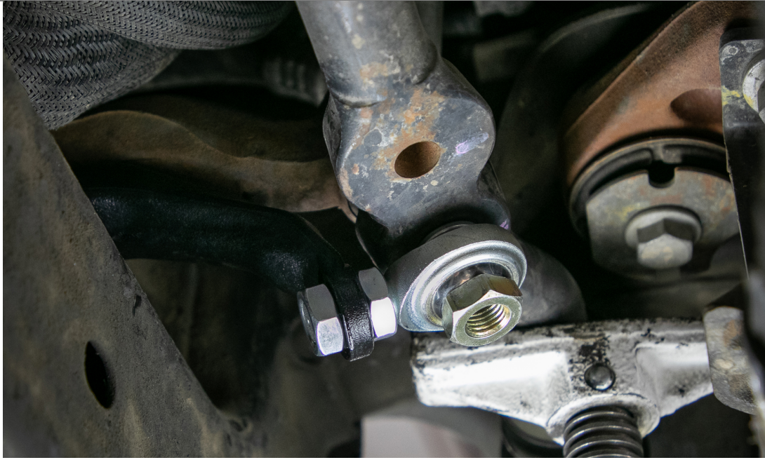
Figure 9: Idler Arm Bracket Installed
