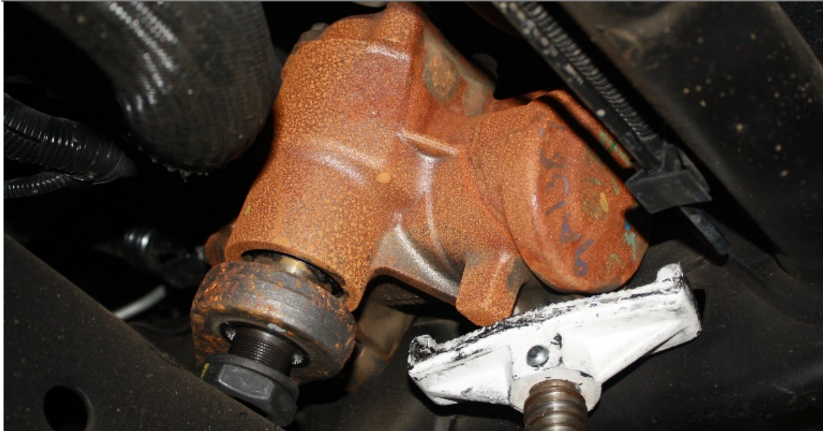
Figure 4: Support the Steering Box with a Jack
