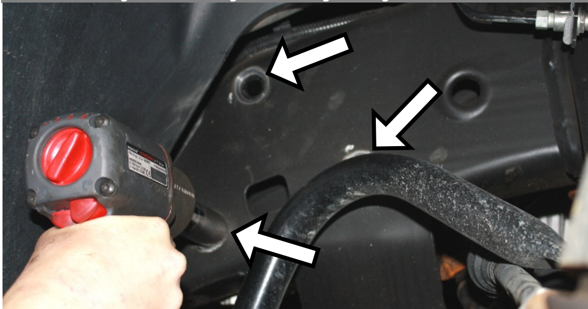
Figure 5: Removing Bolts Holding Steering Box to Frame
