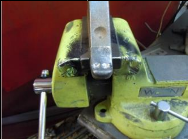
Figure 17: using a drill motor and 1/2" drill bit, drill only 1/8" deep from the tip so create 2 countersink spots.
