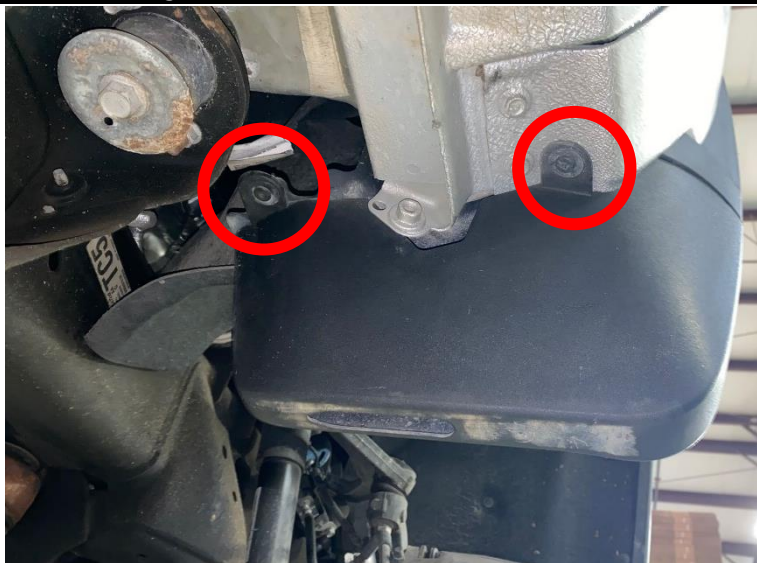
Figure 2: Remove 2 screws under vehicle.
