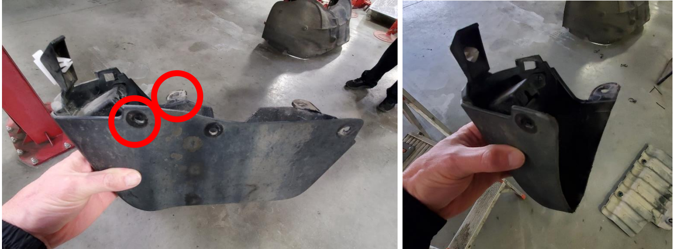
Figure 10: Before and after trimming the mud guard. Do not trim circled holes.
