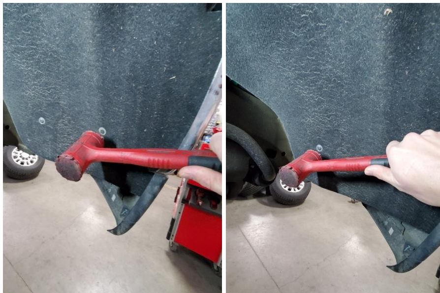
Figure 11: Before and after trimming the mud guard. Do not trim circled holes.
