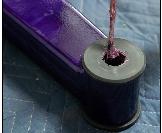
Figure 17: Traction bar bushing grease application.
