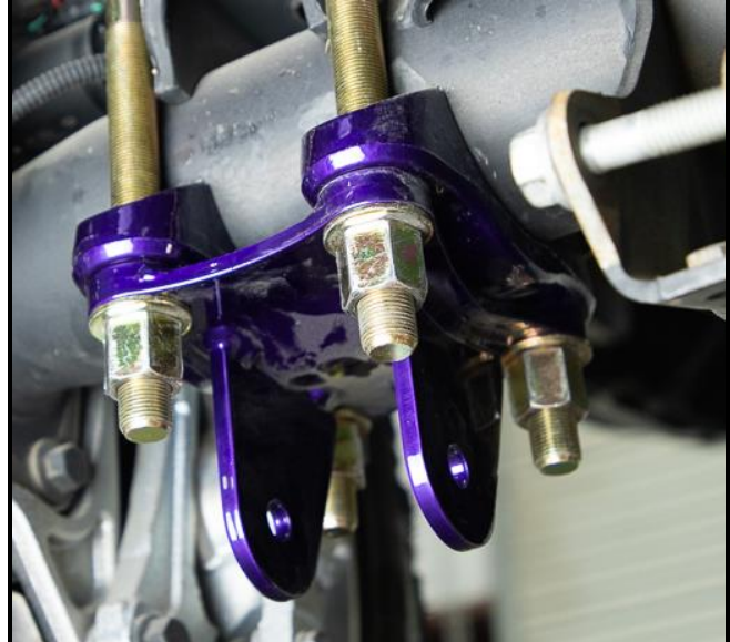
Figure 15: Leaf spring axle bracket installation.
