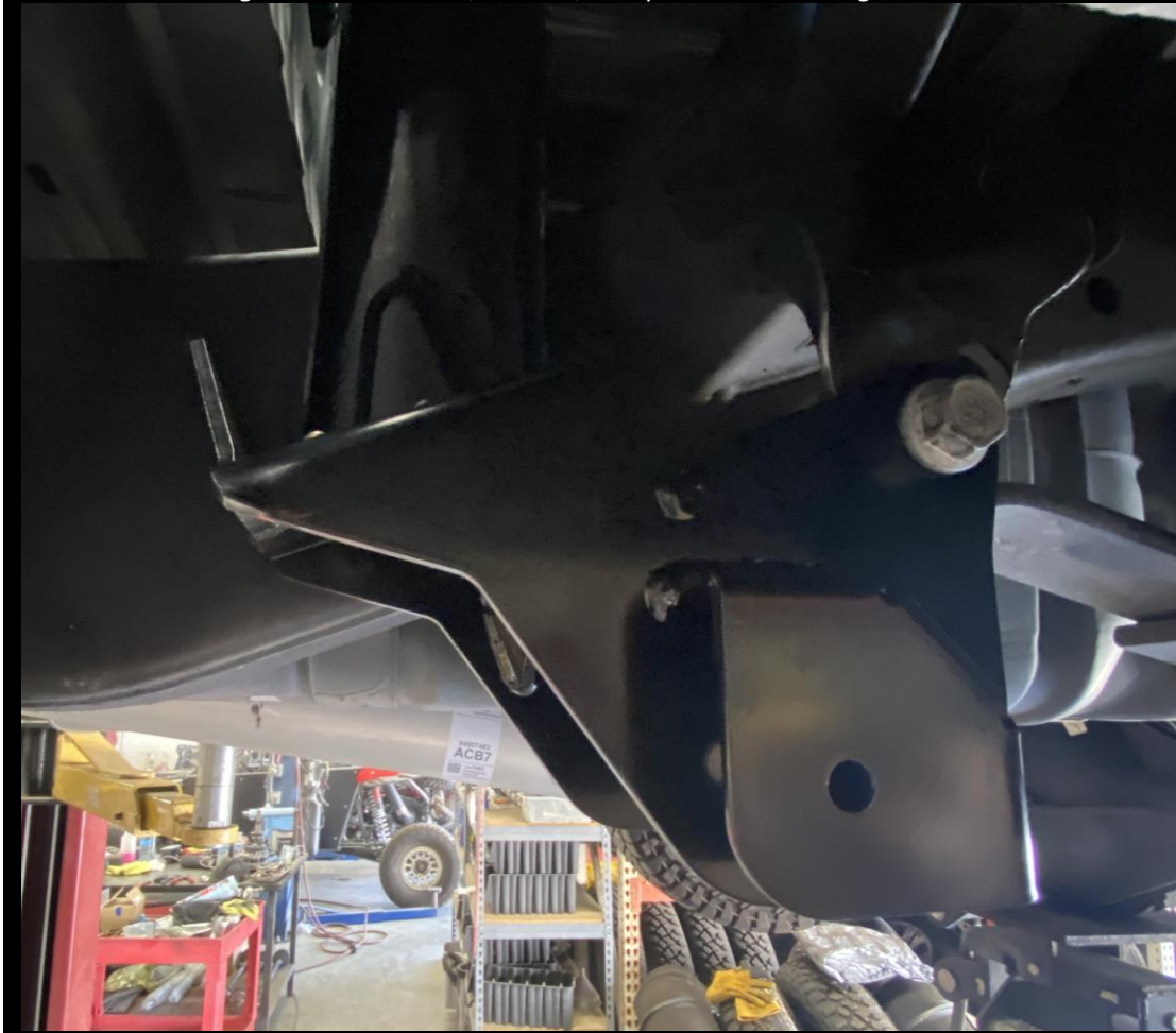
Figure 9: Assembled, welded, and painted mounting bracket.
