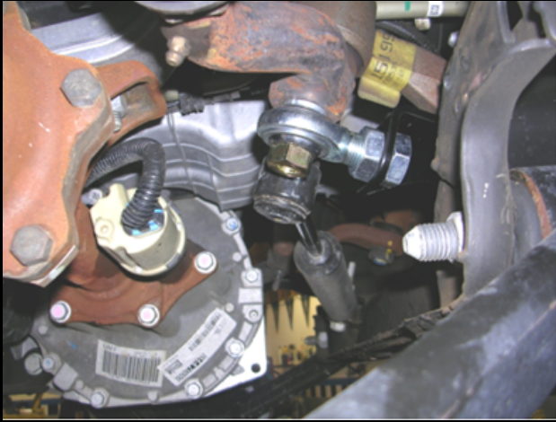
Figure 4: Idler arm bracket installed
