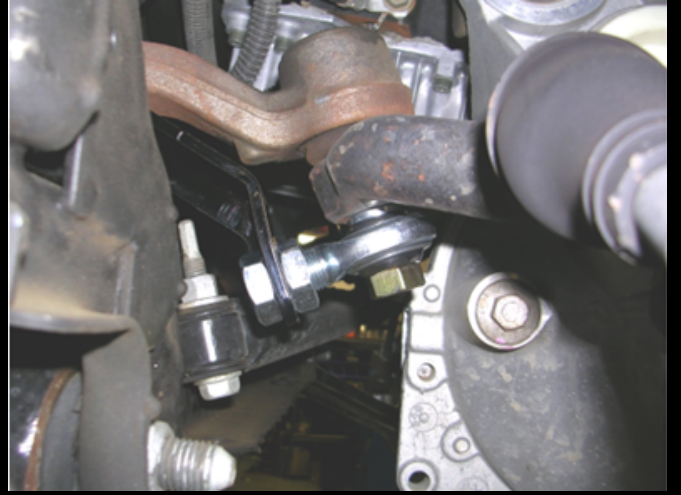
Figure 5: Pitman arm bracket installed
