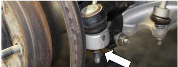
6) Loosen the upper Ball joint/Spindle nut so it's only engaged a couple threads. You will need to smack this junction with a dead-blow hammer to separate the joint; leaving the nut on will ensue the knuckle/arm separation is controlled.
