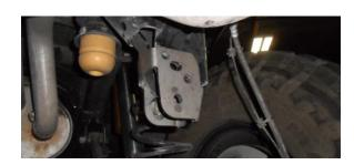
**b.** Install the provided ½" x 2.Bolt and washer in the upper hole of the Carli/Factory Bracket to index the drop bracket.
