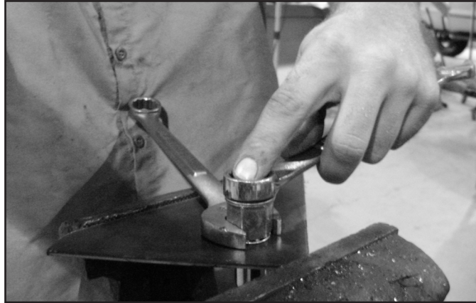
FIGURE 2 - 1/2" RIVET NUT SHOWN
