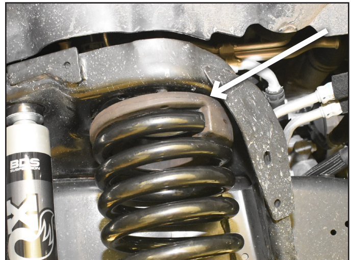
FIGURE 12B PASSENGER'S SIDE - INCORRECT
