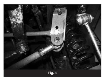
18. With the support tube loosely attached to the track bar bracket on the driver's side, swing it up to the bottom of the passenger's frame rail. Position the end of the tube so that the hole is approximately 5/8" behind the back edge of the existing hole in the frame. Using the hole in the tube as a guide, mark the hole location to be drilled. This hole location will match up with an existing hole in the top of the frame. Lower the tube and drill a 1/2" hole at the mark (Fig 9).
