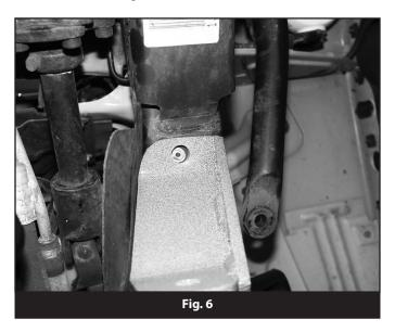
14. With the hole position marked for the track bar bracket, rotate the bracket out of the way and drill a 7/16" hole at the mark. Only drill through the bottom surface of the frame. Attach the track bar bracket to the bottom of the frame (Fig 7) through the new hole with a 7/16" x 1-1/4" bolt, 7/16" SAE washer (BP 753) and provided nut tab (01356). Use Loctite on the bolt threads. Leave hardware loose.
