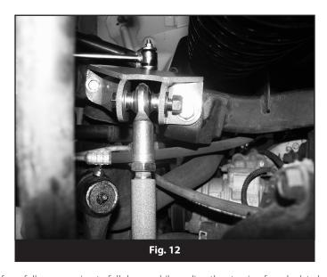
27. Be sure to cycle the suspension from full compression to full droop while cycling the steering from lock to lock. This should identify any clearance issues. Recheck all fasteners after 500 miles.
