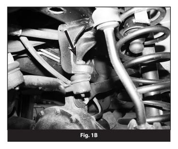
6. Locate the top of the original stabilizer mount on the passenger's side of the axle. Mark from the front edge of the bracket toward the rear ¾" and mark on the top of the bracket (Fig 2). Make a line along the top of the bracket, parallel to the front face at the ¾" marked distance. This will be a reference line for installing the new stabilizer mount/support gusset.
