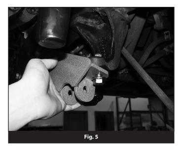
13. Rotate the track bar bracket so that the front end fits flush against the bottom of the frame. The front edge of the bracket should be roughly parallel to the welded edge of the steering box mount. The front outside edge of the bracket should be flush with the outside of the frame. Mark the hole to be drill on the bottom surface of the frame (Fig 6).
