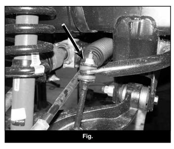
2. Install the sway bar link extension onto the factory sway bar link. Attach the assembly to the sway bar with the factory bushing, cup washers, and 10mm bolts (Bolt pack #654) and Loctite on threads. Tighten bolt until bushings begin to deform. It is NOT necessary to over tighten the bolt.
