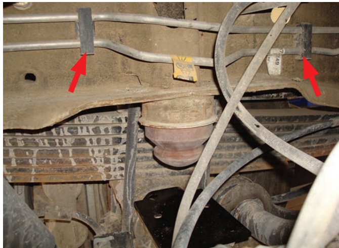
Unbolt and pull the fuel lines away from the frame to gain clearance to drill the holes needed to install the upper bracket.
